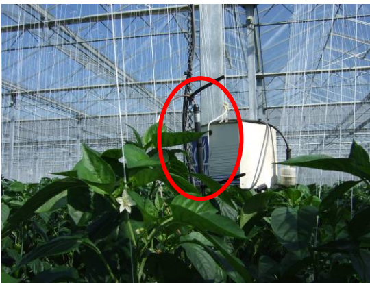
Figure 7. Measuring box with independent temperature and humidity probe (circled)
