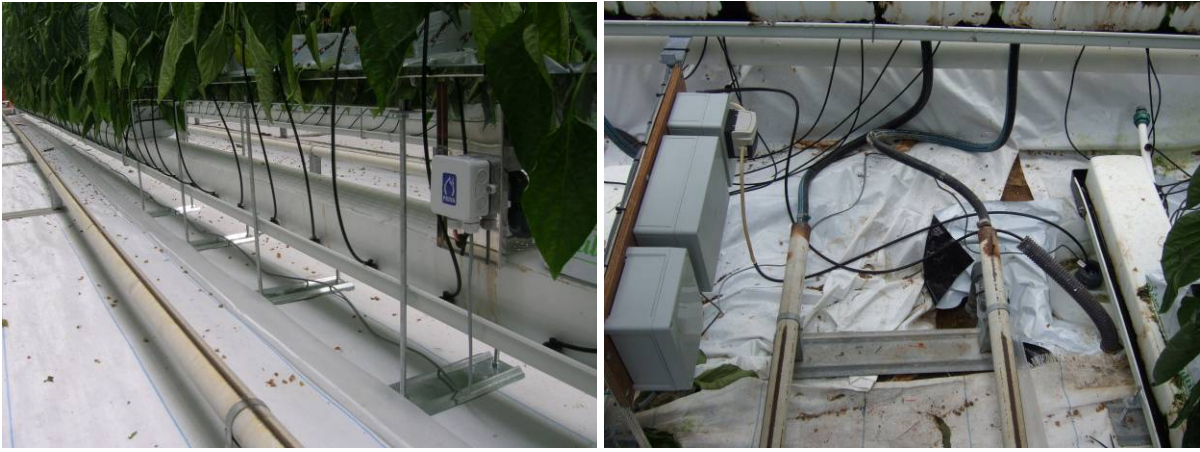
Figure 9. Priva tipping spoon (left) and the end of the Martin Drop drain equipment (right)
